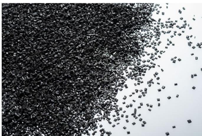
Injection molding granules developed by Kurz from residual and recycled PET material.
