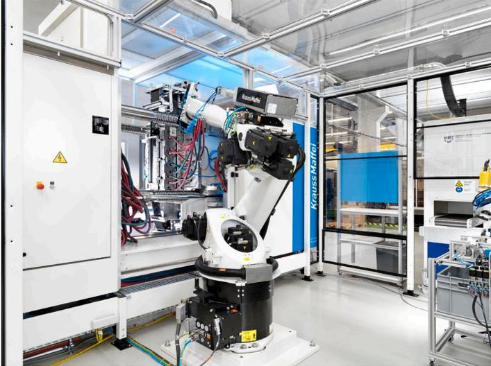
The articulated robot moves the panel to the next process step.
